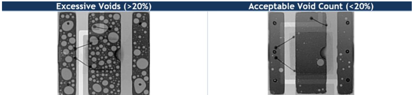
Figure 9, Comparison of good and bad void levels in a solder joint.
