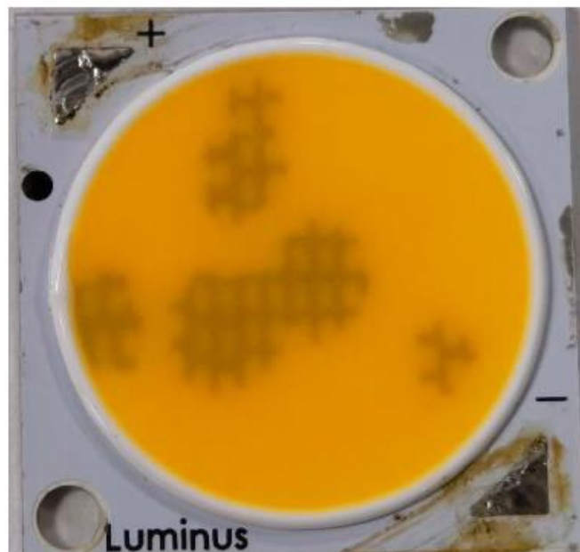
Figure 7 - Example of silver-plated substrate darkening due to storage in an area with an excessive level of sulfur-containing compounds.
