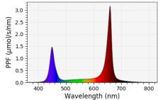
Red-Blue-WW spectrum with 14 SST-10-B ( $450\,\mathrm{nm}$ ) packages, 28 SST-10-DR (660) packages and 14 SST-20-W40H warm white ( $3000\mathrm{K}$ ) packages. The electrical input is 50 Watts at 350 mA drive current and the PPF output is 128 umol/s with a PPF/W of 2.55 umol/J.
