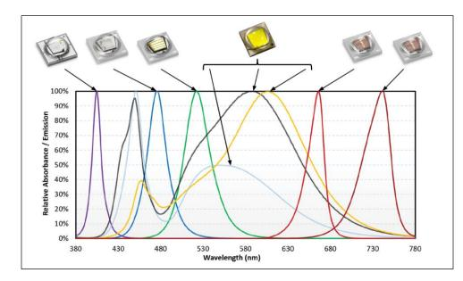
Luminus LEDs span the spectral range needed for horticultural applications. For example, left to right: SST- UV, SST-B, SST-G, SST-W, SST-DR and SST-FR.
