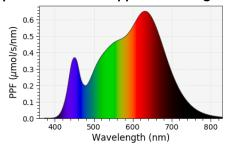
50 SST-20-W40H warm white packages. The electrical input is 52.5 W at 350 mA drive current and the PPF output is 118 umol/s with a PPF/W of 2.26 umol/J.
