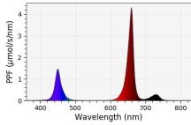
Red-Blue-IR spectrum with 14 SST-10-B (450 nm) packages, 40 SST-10-DR (660) packages and 5 SST-10-FR infrared (730 nm) packages. The electrical input is 49 W at 350 mA drive current and the PPF output is 124 umol/s with a PPF/W of 2.54 umol/J.
