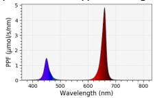
Red Blue spectrum with 15 SST-10-B (450 nm) packages and 45 SST-10-DR (660 nm) packages. The electrical input is 49 Watts 350 mA drive current and the PPF output is 135 umol/s with a PPF/W of 2.76 umol/J.
