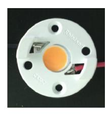
Fig. 10 Proper Centering of LES in Holder
