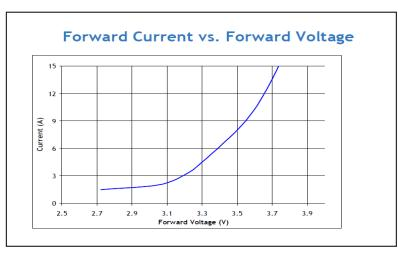
Figure 3: Typical I-V curve of a Big Chip LED
