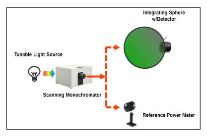
Figure 2: Substitution method of calibration
