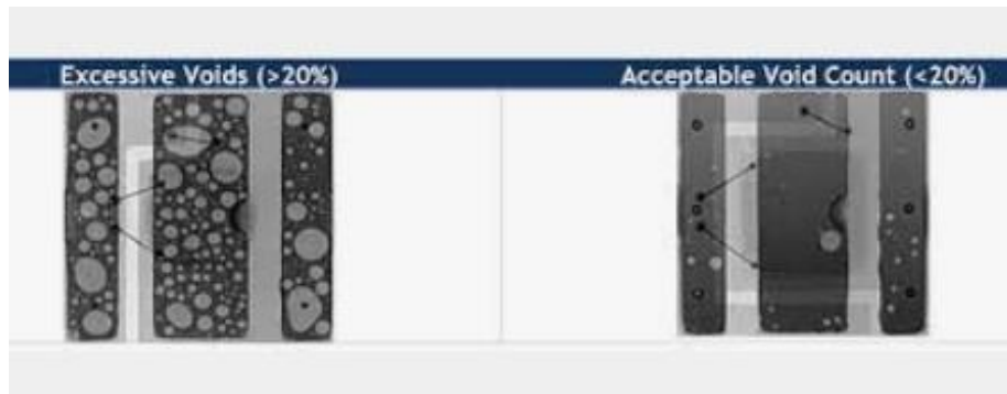
Figure 10. Comparison of good and bad void levels.
