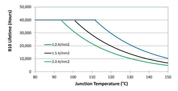
Note 8 Lifetime defined as time to 70% of initial intensity. Based on preliminary lifetime test data. Data can be used to model failure rate over typical product lifetime.
