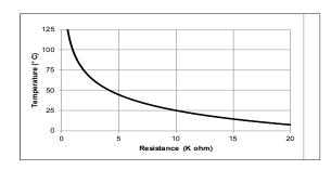
The thermistor used in CBT-120 devices mounted on coreboards is from Murata Manufacturing Co. The global part number is NCP18XH103J03RB. Please see http://www.murata.com/ for details on calculating thermistor temperature.
