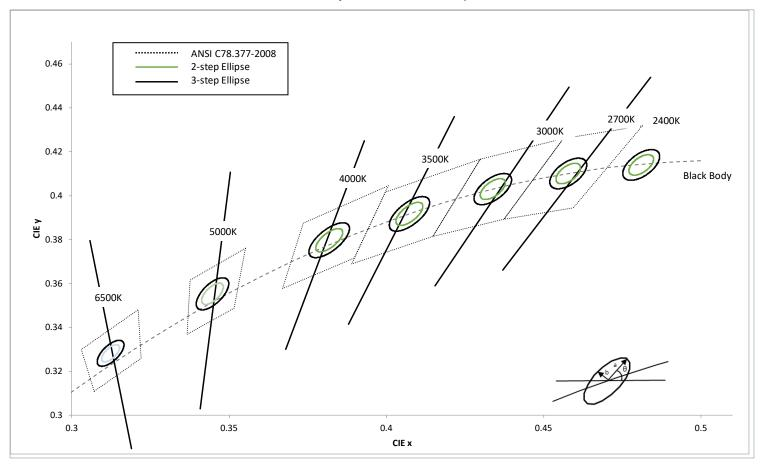
The following tables describe the chromaticity bin center points, the orientation angle for the MacAdam ellipse ( $\theta$ °), and the maximum radii for the ellipses. The ANSI Bin is provided for reference.
