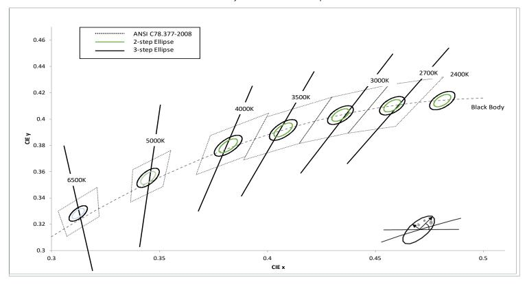
The following tables describe the chromaticity bin center points, the orientation angle for the MacAdam ellipse ( $\theta$ °), and the maximum radii for the ellipses. The ANSI Bin is provided for reference.
