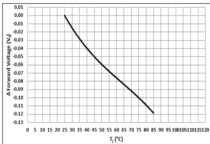
V f vs. T j \Delta V_f = V(T_j) - V(85^\circ\text{C}) Single Pulse 20ms I f = 1A; White
