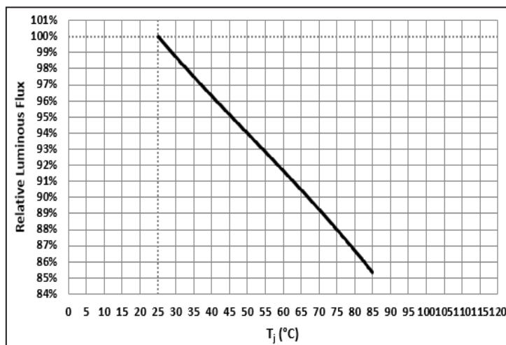
Relative Luminous Flux vs. T_j \phi_v/\phi_v(85^\circ\text{C}) Single Pulse 20ms I_f = 1\text{A} ; White
