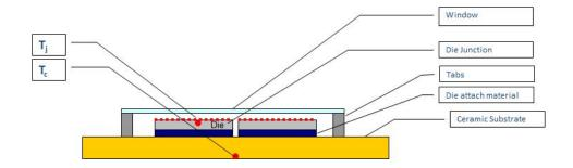
Thermal resistance junction to case, R  $_{th(j-c)\_real} = 1.0$  °C/W (typ.),(All chips operated simultaneously) Thermal resistance junction to case, R  $_{th(j-c)\_electrical} = 0.8$  °C/W (typ.) (All chips operated simultaneously)
