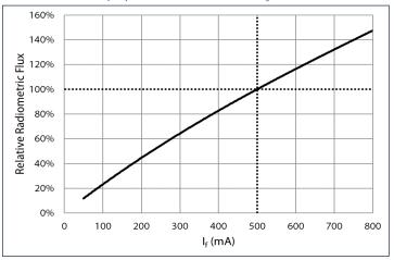
Temperature:  $\varphi_{r}/\varphi_{r}(25^{\circ}\text{C})$ , 20 ms pulse,  $I_{r}$  = 500 mA
