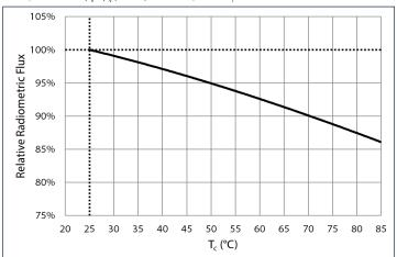
Temperature:  $\Delta V_f = V(T_c) - V(25^{\circ}C)$ , 20 ms pulse,  $I_f = 150$  mA
