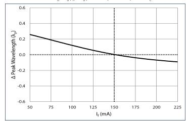
Forward current:  $\Delta \lambda_d = \lambda_d (I_f) - \lambda_d (150 \text{ mA})$ , 20 ms pulse,  $T_c = 25^{\circ}\text{C}$
