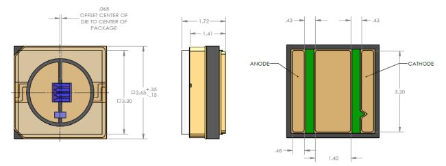
NOTES: 1. DIMENSIONS ARE IN MILLIMETERS. 2. TOLERANCES ±0.20MM. UNLESS SPECIFIED.
