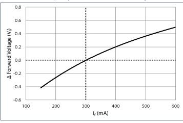
Temperature:  $\Delta V_f = V(T_c) - V(25^{\circ}C)$ , 20 ms pulse,  $I_f = 300$  mA
